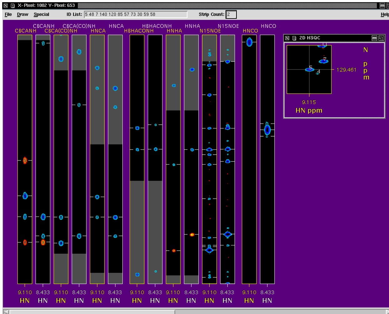
Figure 1.8. A prototype NMRWish TCL application for browsing through strips from related amide-detected 3D experiments, and automatically suggesting which strips might be the next or previous ones in the sequential assignment. Strips from comparable spectra are extended automatically by refolding the data so they can be displayed with uniform chemical shift ranges where needed; the portions of the data which have been extended redundantly this way are shaded in gray. In the example show here, a series of related strips from two different ^1\text{H}/^{15}\text{N} positions are displayed. The inset at upper right displays the corresponding location from a 2D ^1\text{H}/^{15}\text{N} correlated spectrum for the first set of strips being viewed.
